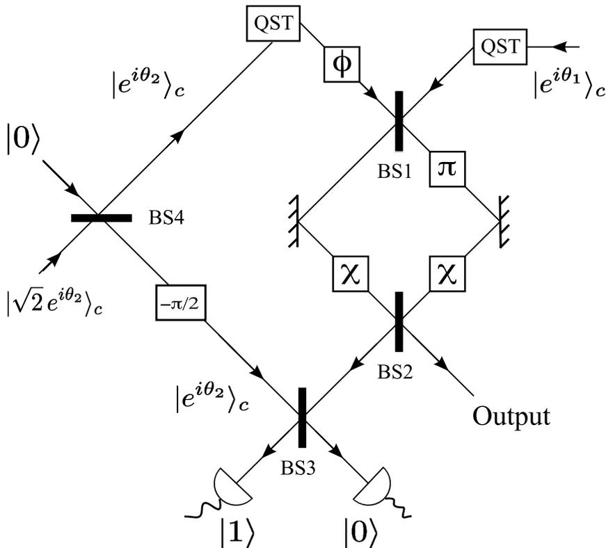
FIG. 6: The full scheme for demonstrating interference between a single particle and the vacuum as given in Figure 6(b). Importantly, as discussed in the text, the phase of the input to the QST scheme on the left and the input to the which-way wash-out scheme at BS3 have their phases fixed. This is achieved by creating them from a common source at BS4.
