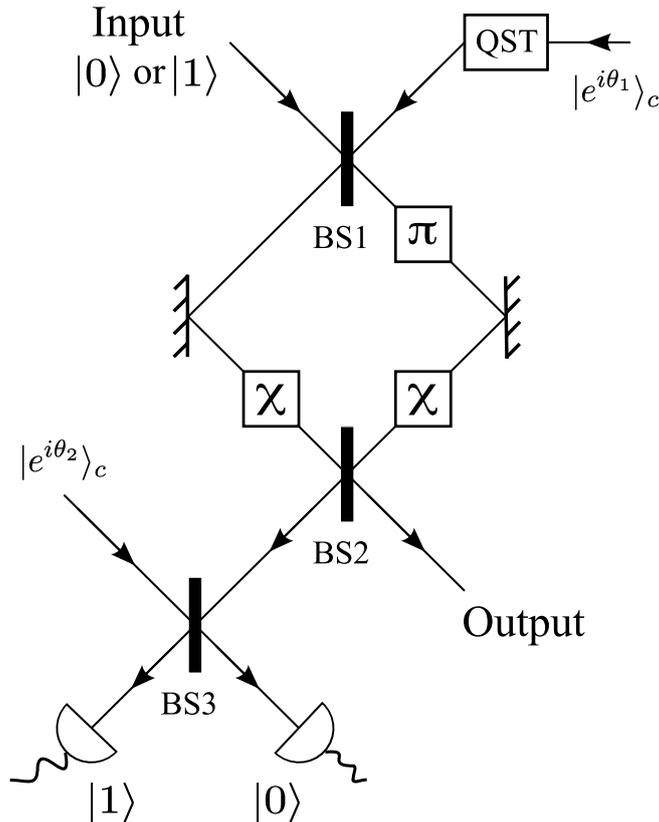
FIG. 3: The Hadamard gate scheme. This consists of three 50:50 beam splitters (BS1, BS2, and BS3), two nonlinearities ( $\chi$ ), a  $\pi$  phase shift ( $\pi$ ) and conditional measurements made at the outputs of BS3. It also makes use of the quantum state truncation scheme shown in Figure 2. The overall transformation that this interferometer performs is given by Equations (24) and (25).
